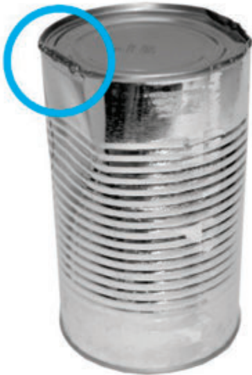
Dented at junction of side and end
