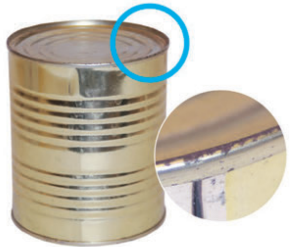
Pitted rust or leaking
